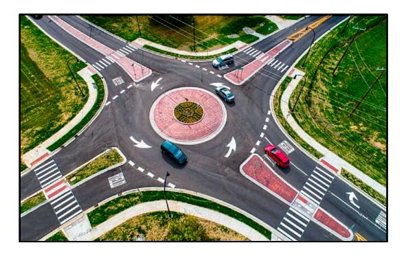
Affordable Compact and Mini-Roundabouts are being implemented by state and local public agencies due to their low cost, quick delivery, reduced vehicle speeds, and ability to prevent up to 90% of severe crashes.
