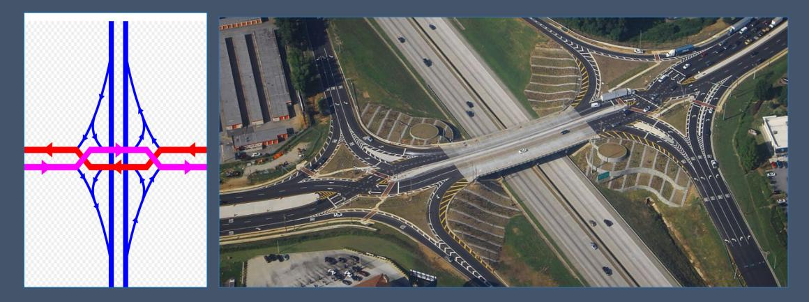
aka *Double Crossover* interchange featuring signals to control only through traffic along the local street or highway
